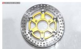
**Gambar 1. Cakram Motor (gridoto.com)**
